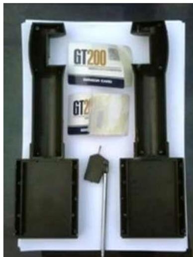
*Figure 2: These devices, as sold, were only empty boxes that contained no electronic components.*
