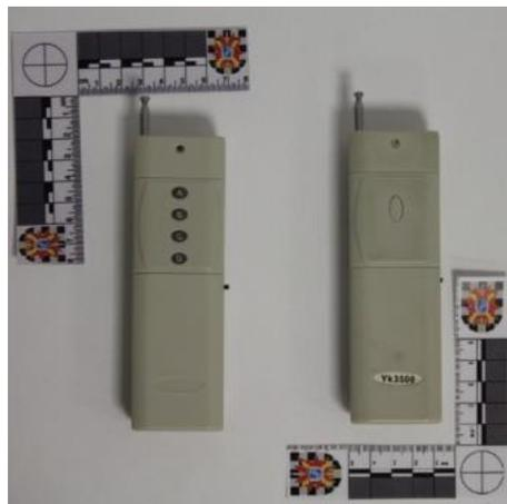
Figure1: Most common RFT-2 transmitters
